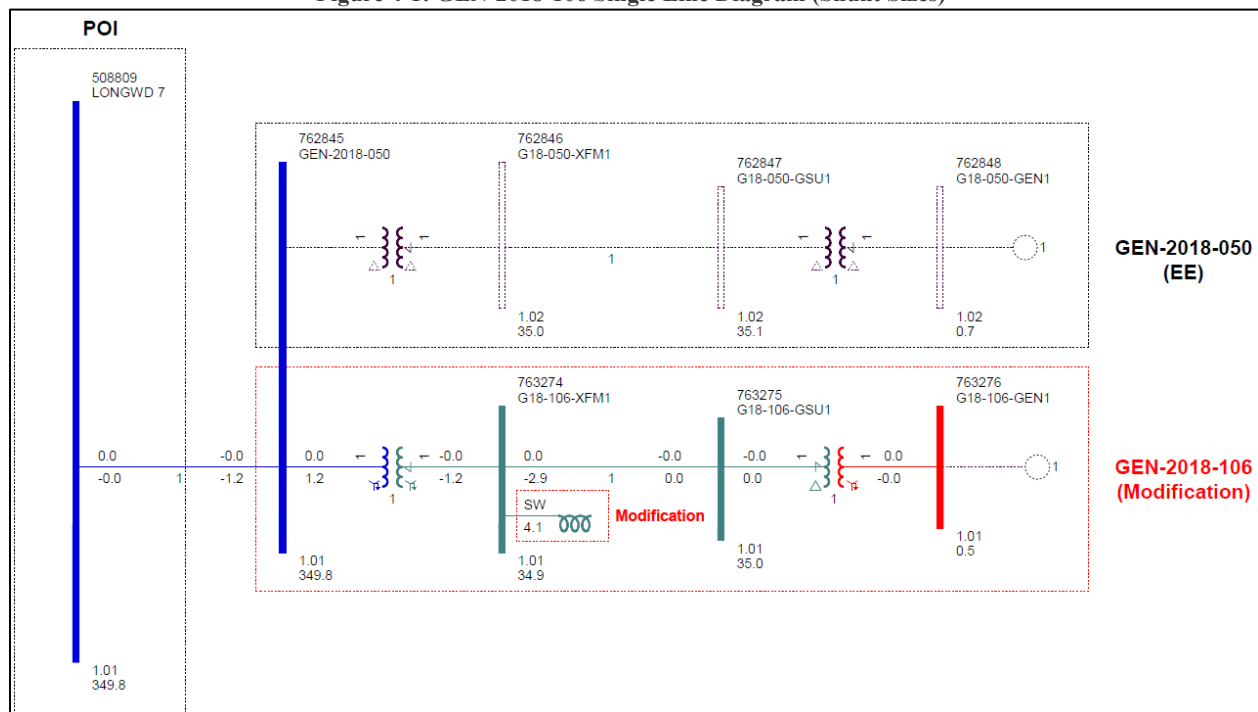
Figure 4-1: GEN-2018-106 Single Line Diagram (Shunt Sizes)
