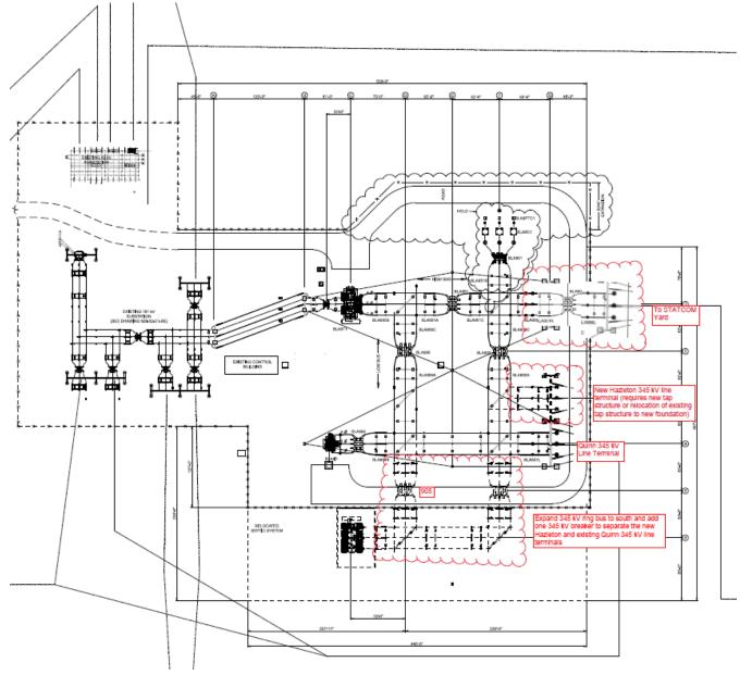
Black Hawk Substation: Expansion to Add One 345 kV, 100 MVAR STATCOM
