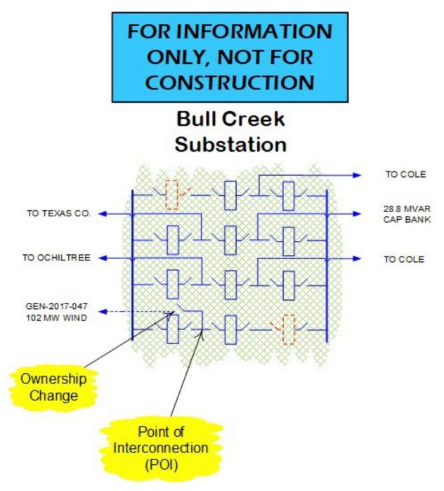
Figure A-3: Point of Interconnection & Change of Ownership Elevation (Typical) \*DIAGRAMS ARE NOT FOR CONSTRUCTION PURPOSES\*
