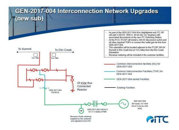
Figure 1 GEN 2017-004 Interconnection Substation One Line
