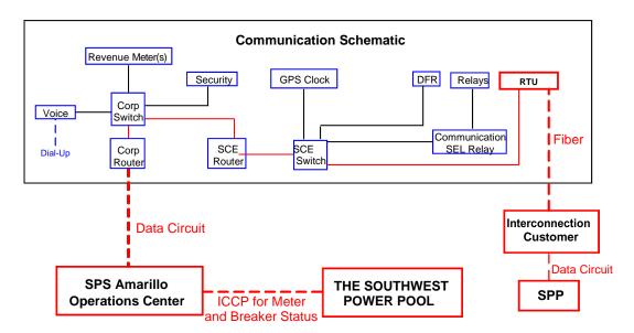
IC shall be responsible for providing the fiber optic communication circuit installed in the overhead transmission line static wire from the customer substation to the SPS substation for protective relaying and for transmitting metering and status data to SPS. Utilizing this fiber optic connection, SPS will establish a direct connection to the IC's RTU.
