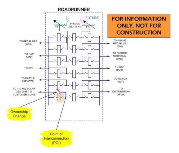
Figure A-3 Point of Interconnection & Change of Ownership Elevation (Typical)
