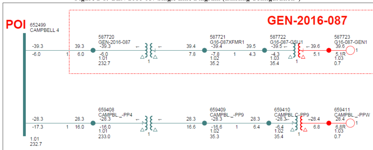
Figure 2-1: GEN-2016-087 Single Line Diagram (Existing Configuration*)
