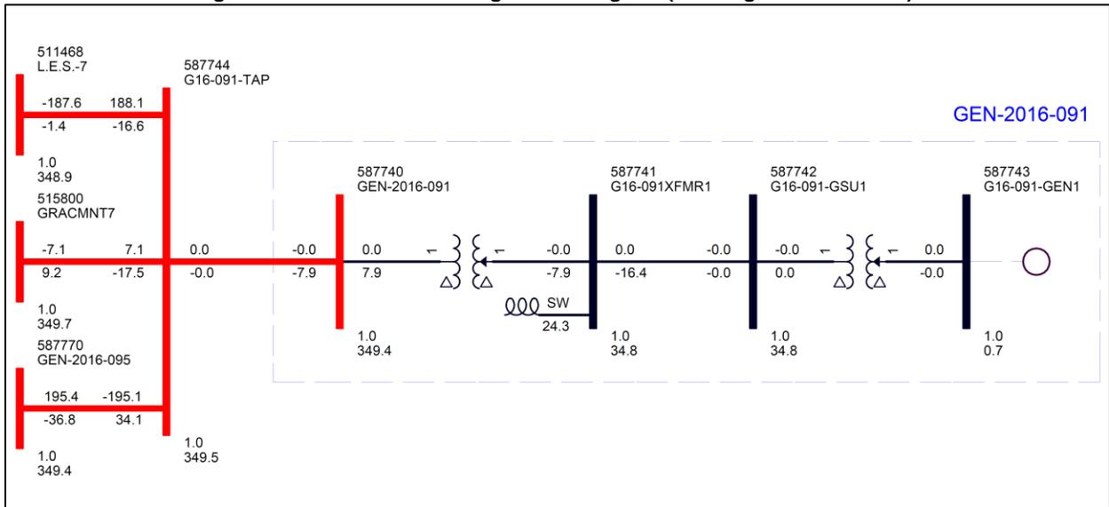
Figure 4-2: GEN-2016-091 Single Line Diagram (Modification Shunt Reactor)
