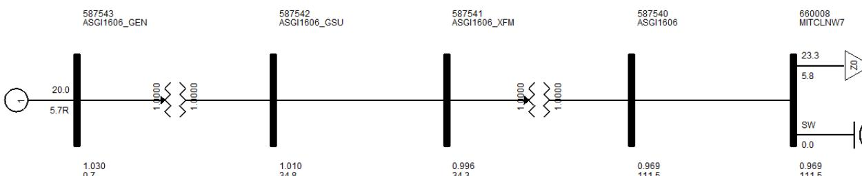
The POI for ASGI-2016-007 Interconnection Customer connects to the Affected System Mount Vernon 69kV substation in Aurora County, South Dakota. Figure 3 depicts the one-line diagram for the POI and the Interconnection Request(s).
