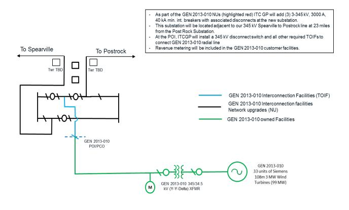
Figure 1 GEN-2013-010 ITCGP Interconnection Substation One Line
