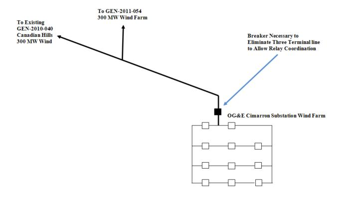
Figure 1: Gen 2011-054 Facility and Proposed Interconnection Configuration
