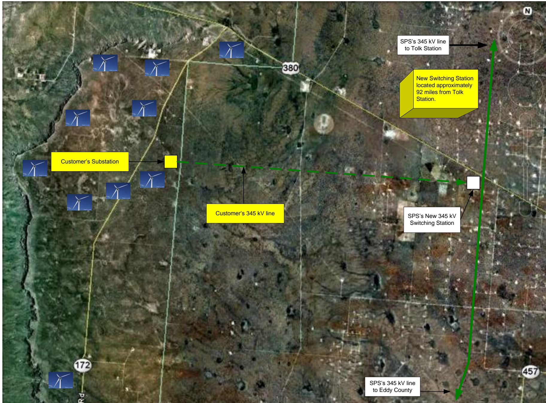
Figure A- 1 Approximate location of proposed SPS Switching Station and Wind Farm Facility
