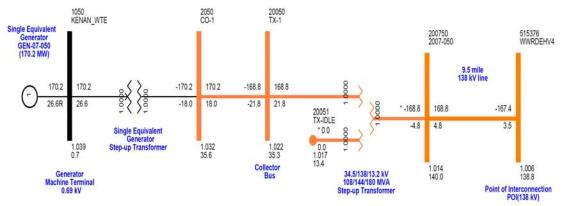
Figure 4-1: one-line diagram for GEN-2007-050 project
