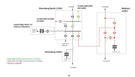
Figure 1: GEN-2006-044N Facility and Proposed Interconnection Configuration
