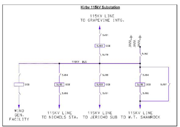
Figure 1-2: Schematic diagram for the interconnection of GEN-2005-021
