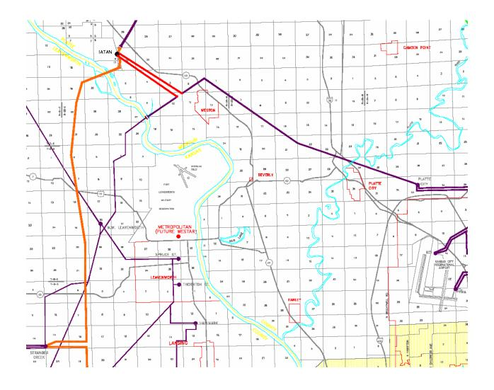
Proposed new 161kV line additions (in red) for new 900 Mw generating unit at latan.
