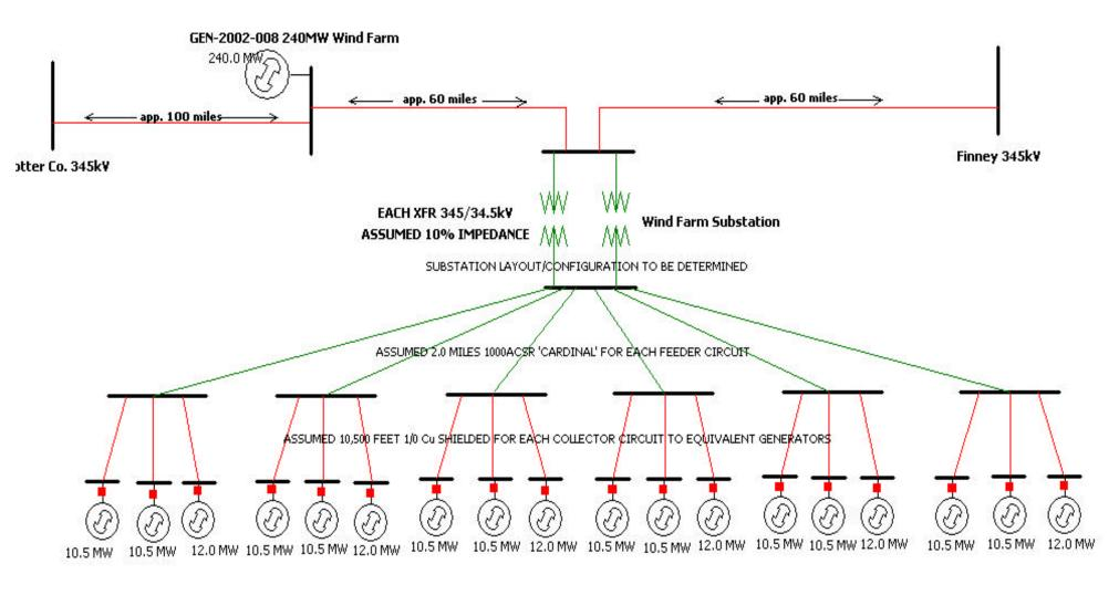
EACH GENERATOR IS EQUIVALENT TO EITHER 7 OR 8 WIND TURBINES (1.5MW EACH) GENERATOR EQUIVALENTS INCLUDE PAD MOUNT XFR CHARACTERISTICS
