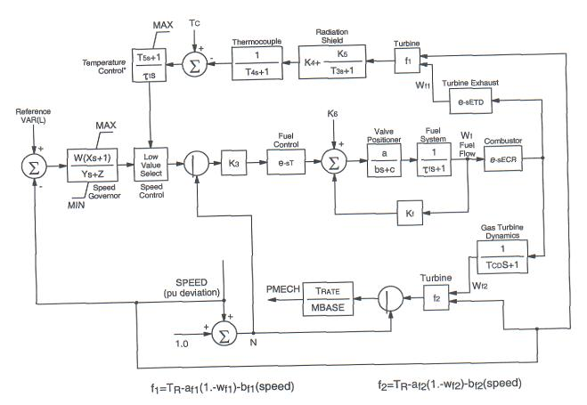
\*Temperature control output is set to output of speed governor when temperature control input changes from positive to negative.
