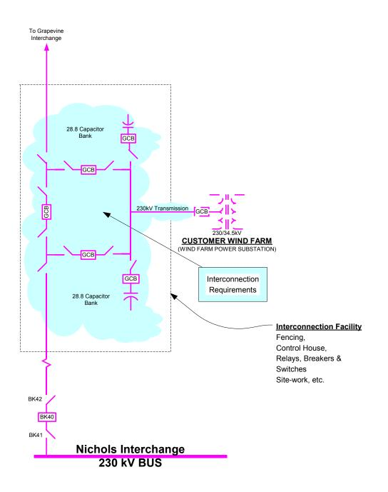
Figure 1, One-line Diagram of the 230 kV Interconnection Facility.
