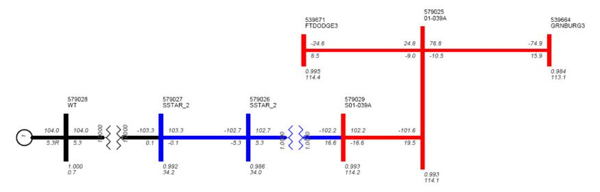
Figure 3-1. Power Flow One-line for GEN-2001-039A and adjacent equipment
