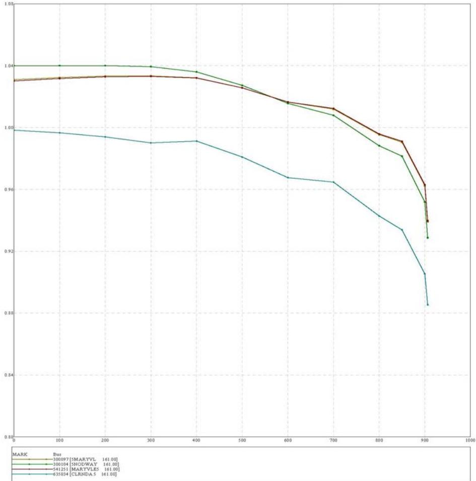
**Figure 1. Voltages for Wind Farm Generation for the loss of the Wind Farm – Midway 161kV line**
