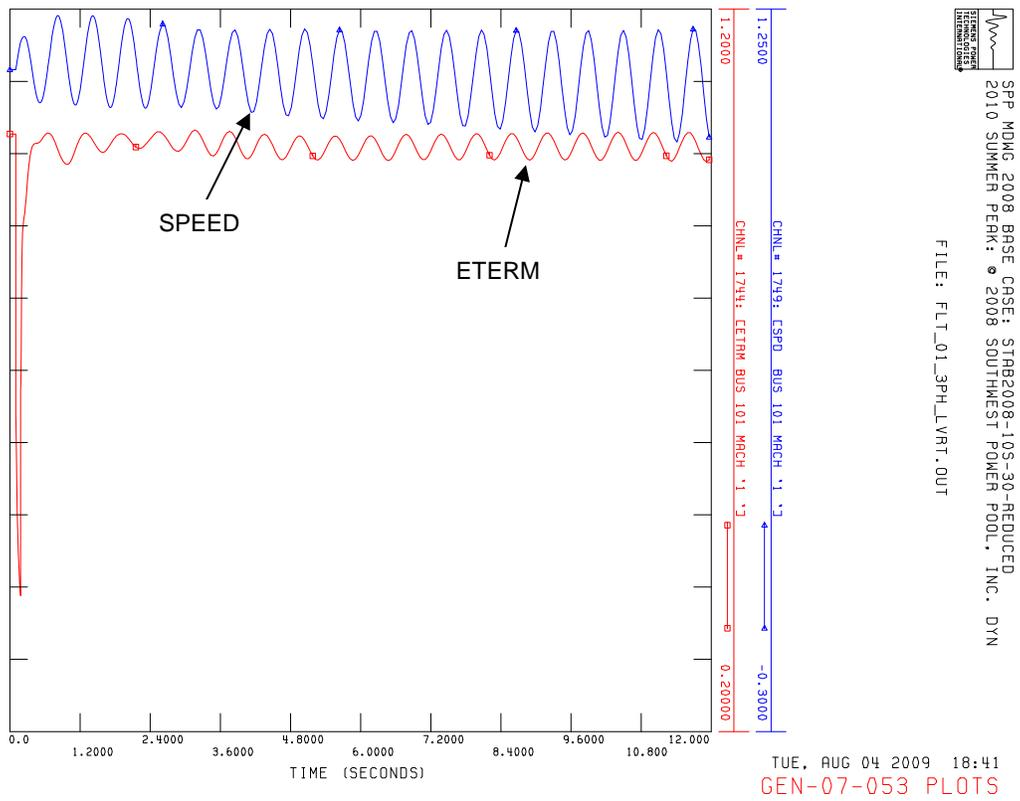
Figure 6-3 Voltage recovery following FLT01-3PH\_LVRT (summer peak)
