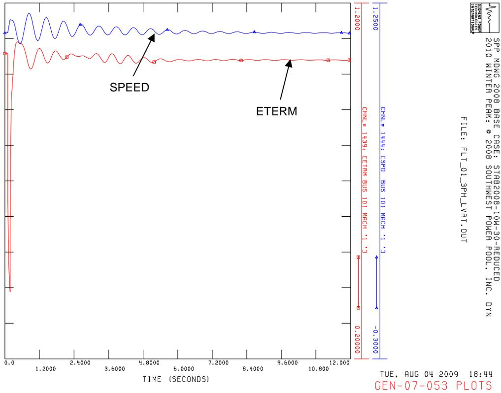
**Figure 7-4** Voltage recovery after FLT01-3PH\_LVRT (winter peak updated model)
