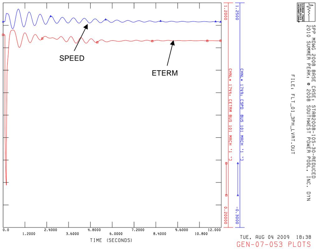
Figure 7-3 Voltage recovery after FLT01-3PH\_LVRT (summer peak update model)
