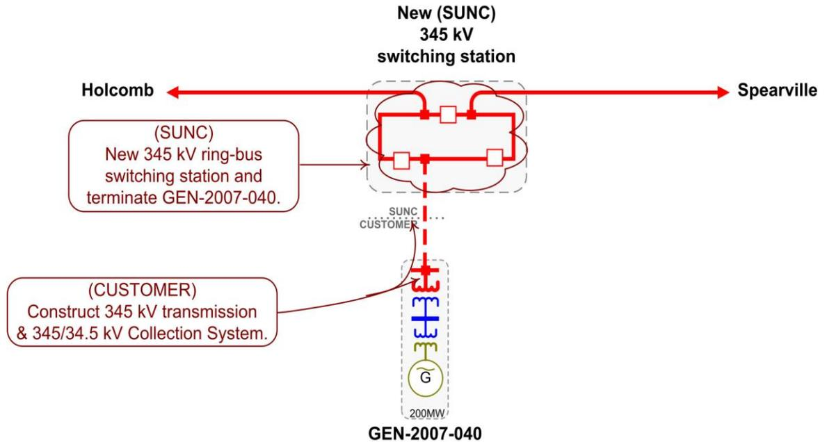
Figure 1: GEN-2007-040 Facility and Proposed Interconnection Configuration
