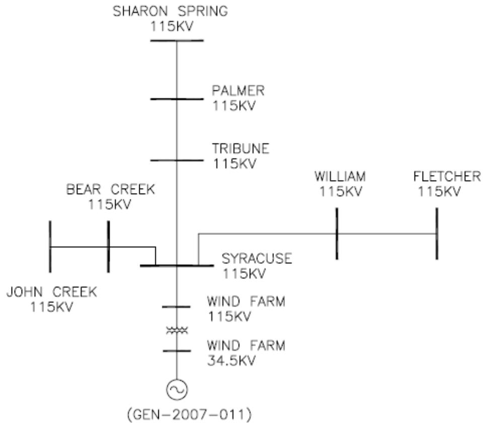
Figure 1: System One Line Diagram near GEN-2007-011
