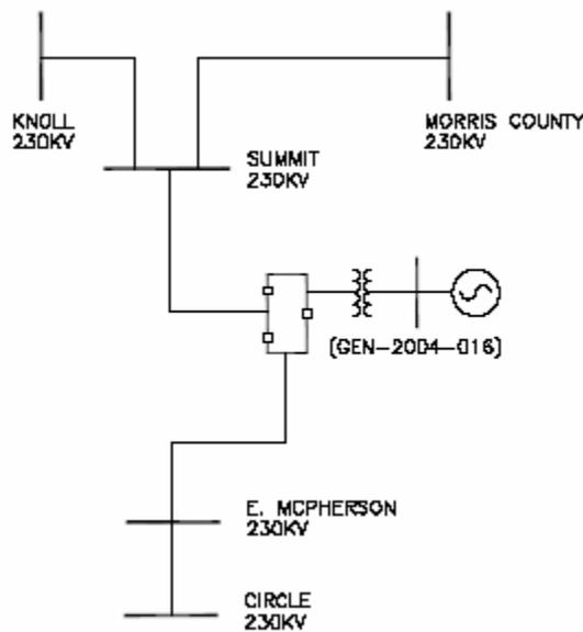
Figure 1 : System One Line Diagram near GEN-2004-016
