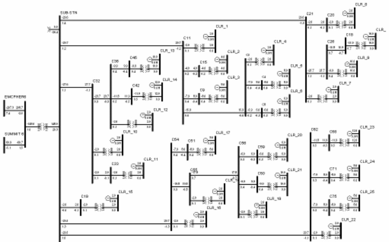
Figure 2 : 100% Power Flow Base Case for GEN-2004-016
