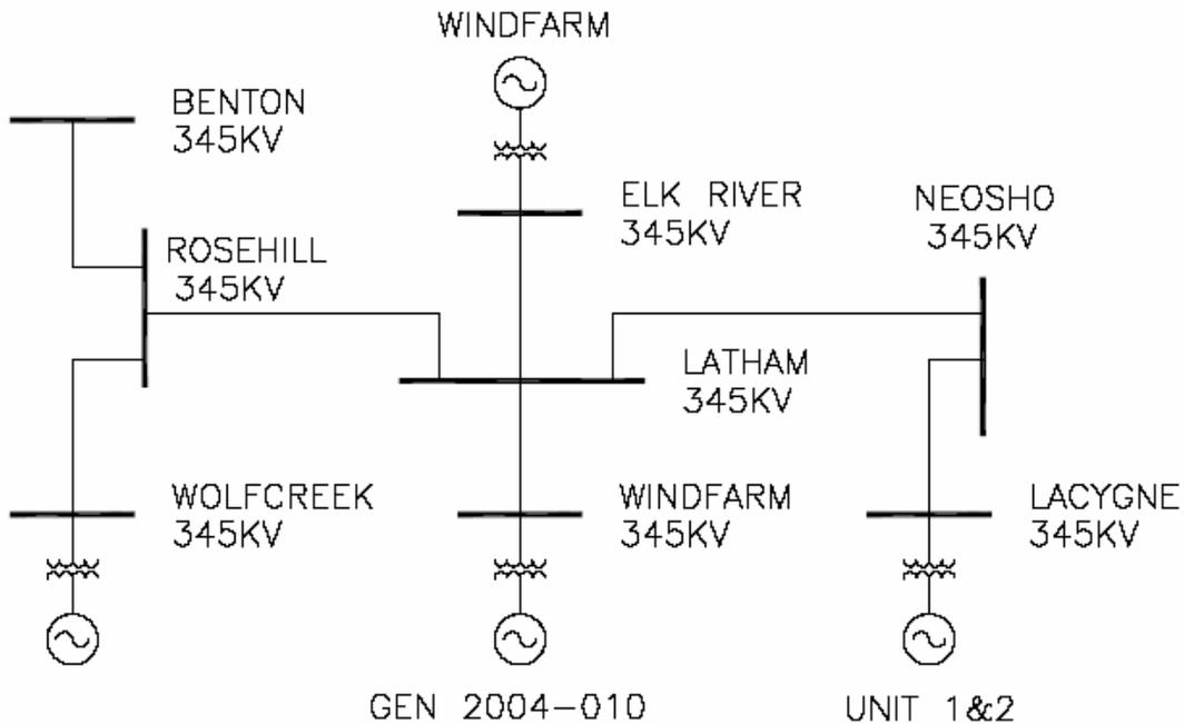
Figure 1: System One Line Diagram near GEN-2004-010
