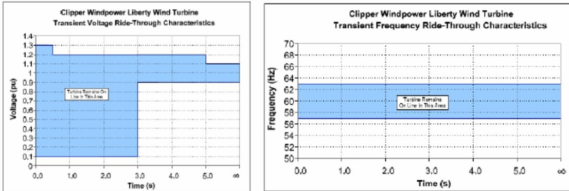
Figure 3: Protective Settings for voltage and frequency.
